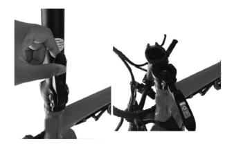
**2-** Open folding apparatus place on lower section of handlebar and fold handlebar towards down to front wheel.
