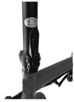
**3-** When your vehicle's folding apparatus and handlebar folding apparatus are open, prepare your vehicle and handlebar for folding.
